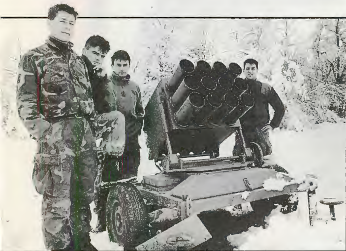
MUP trainees stand in snow by 12-round variant of Yugo Plaman 128mm multiple rocket launcher. When winter offensive comes, it will be cold, wet, bitter: At least these gunners don't have to fire their weapons from the prone.
